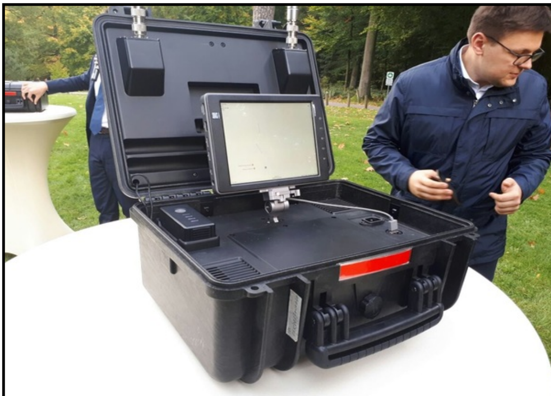
Figure 1. DJI ID AeroScope ground unit (photo by Gareth Corfield)
